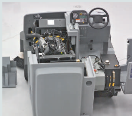
The Nilfisk NoTools™ system makes service extremely easy. The 5-sided access to engine and hydraulic components saves you valuable time and keeps down the service cost
