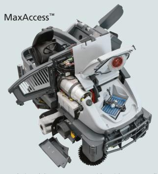
We designed the CS7010 to provide quick access to all vital systems for easier inspection and maintenance
