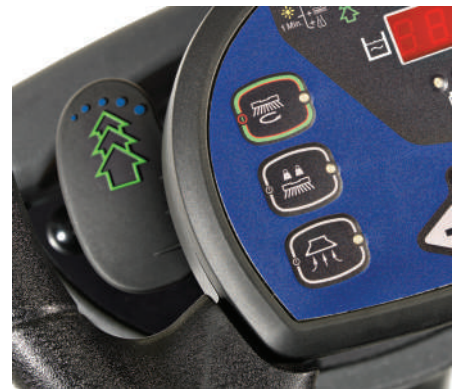
One paddle activates & de-activates the Ecoflex system
